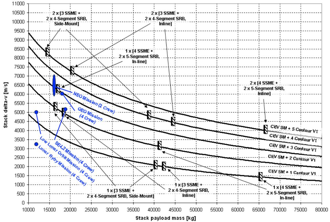
Figure 5: Results of the integrated performance analysis for configurations based on the Centaur V1 upper stage
