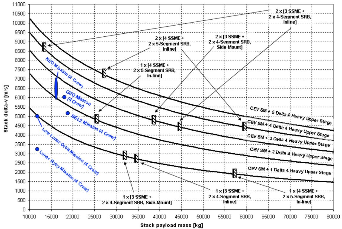
Figure 4: Results of the integrated performance analysis for configurations based on the Delta IV heavy upper stage
