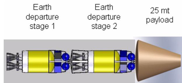
Figure 1: Earth departure stack with two 25 mt LOX / LH<sub>2</sub> propulsion stages per 25 mt payload
