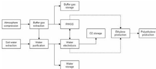
**Figure 7: Alternative ISRU architecture for the initial Mars toehold with RWGS instead of zirconia electrolysis**
